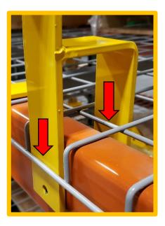
(2) Slide bolt through the holes on the legs of the Pallet Beam Stop. Secure the bolt in place with the nylon hex nut. Tighten nut until Pallet Beam Stop is snug and securely in place.
